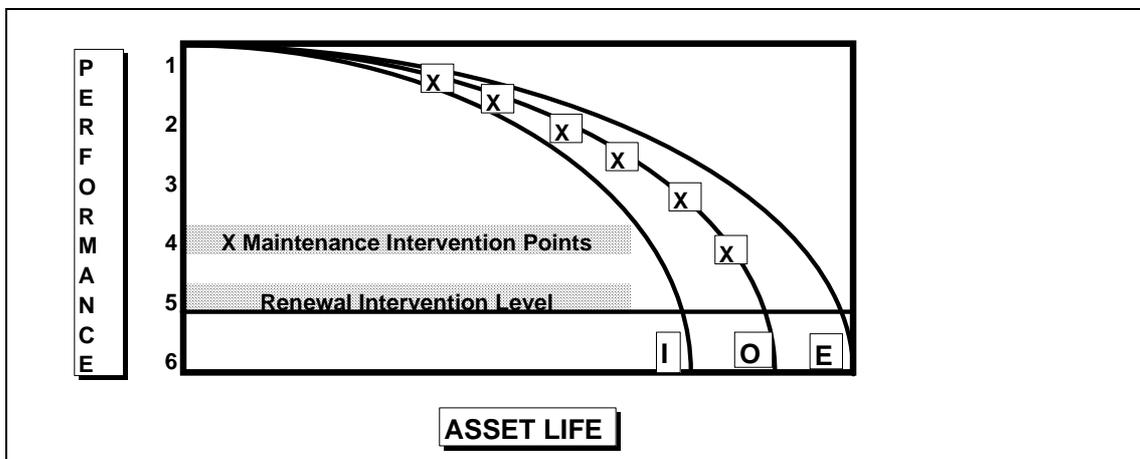
Maintenance Level I (inadequate) O (Optimal) E (excessive)
